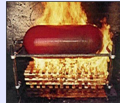
Structural composites industry, fire proof cylinders
