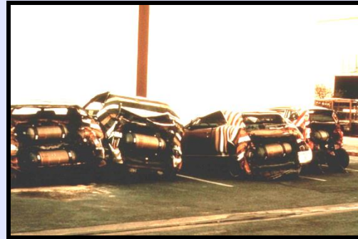
10 ...17....23...30m drops ...no leakage!!
