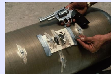
CNG Cylinder Severe Abuse Test 1983
