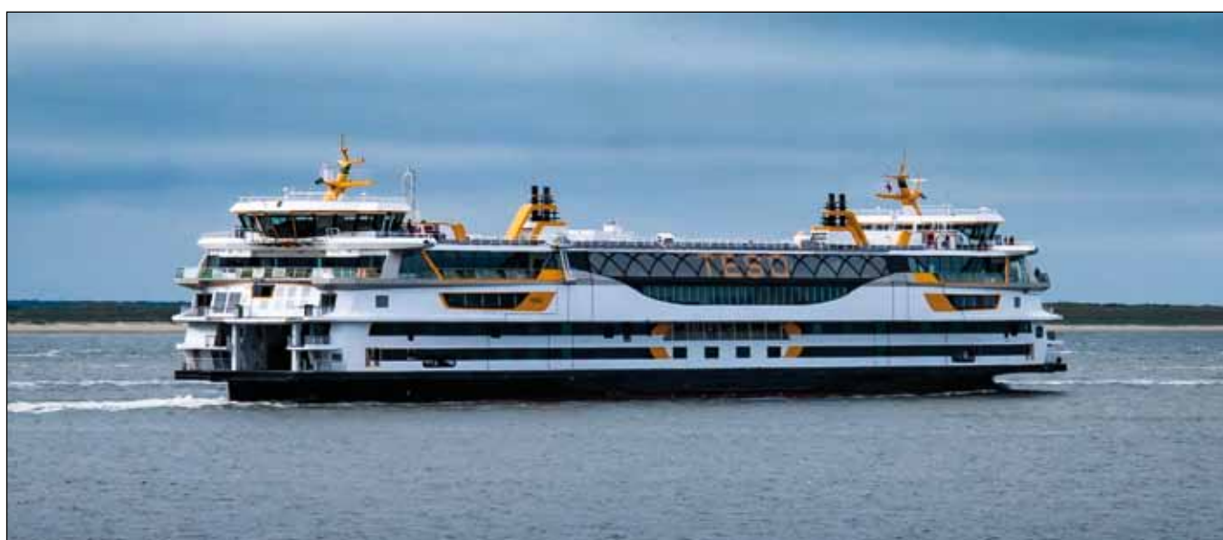
The MS Texelstroom, operated by Dutch shipping company TESO, became the first ferry in Europe to run on CNG in July 2017, reducing emissions and increasing fuel efficiency. The ferry connects the island of Texel with the mainland at Den Helder.
